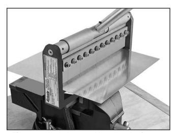
Figure 6. Workpiece positioned under fingers.
